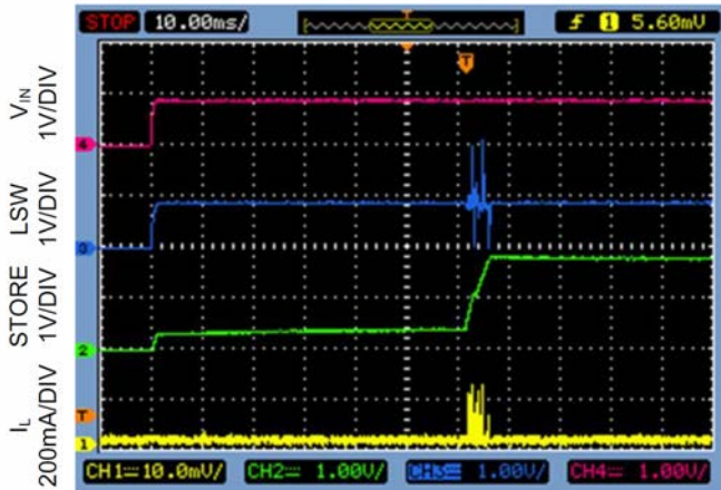
Startup : Circuit A with R_{IN}=10\Omega V_{IN}=0.9V , STORE=1.8V, I_{STORE}=0.18\mu A
