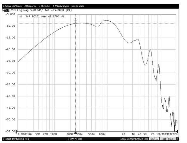
Figure 8-32. Off-State Data-Switch Isolation vs Frequency (TPS25832-Q1)
