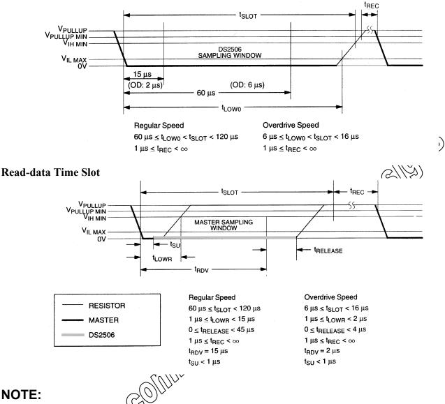
**NOTE:** For read-data time slots the optimal sampling point for the master is as close as possible to the end time of the  $t_{RDV}$  period without exceeding 15 µs for regular speed or 2 µs for overdrive speed. For the case of a read-one time slot, this maximizes the amount of time for the pull-up resistor to recover the line to a high level. For a read-zero time slot it ensures that a read will occur before the fastest 1-Wire device releases the line  $t_{RELEASE} = 0$ .
