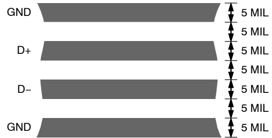
Figure 23. Typical Arrangement of Signal Tracks
